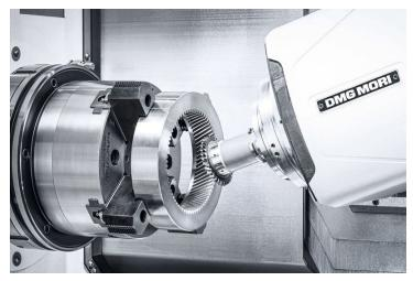
Since the merger of Mori Seiki and DMG in 2015, DMG Mori has topped the list of the Top 100. In the image: A B-axis with a 90 Nm powerful turn-mill spindle replaces the tool turret on the CLX 550 TC.
